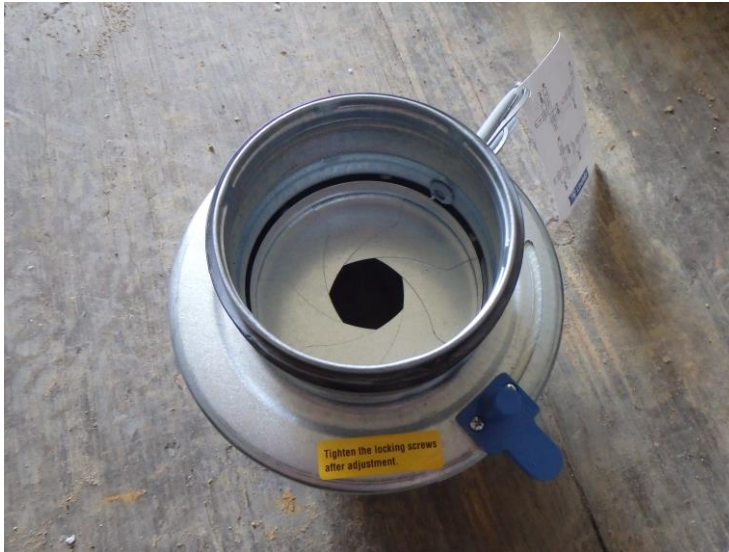
Fig. 5.7 Picture of the adjustable orifice plate: DIRU 100.
