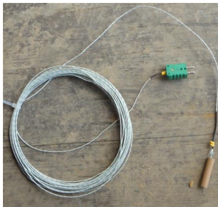
Fig. 5.5 Picture of one thermocouple with the plug at one end and the weld at the other end.
