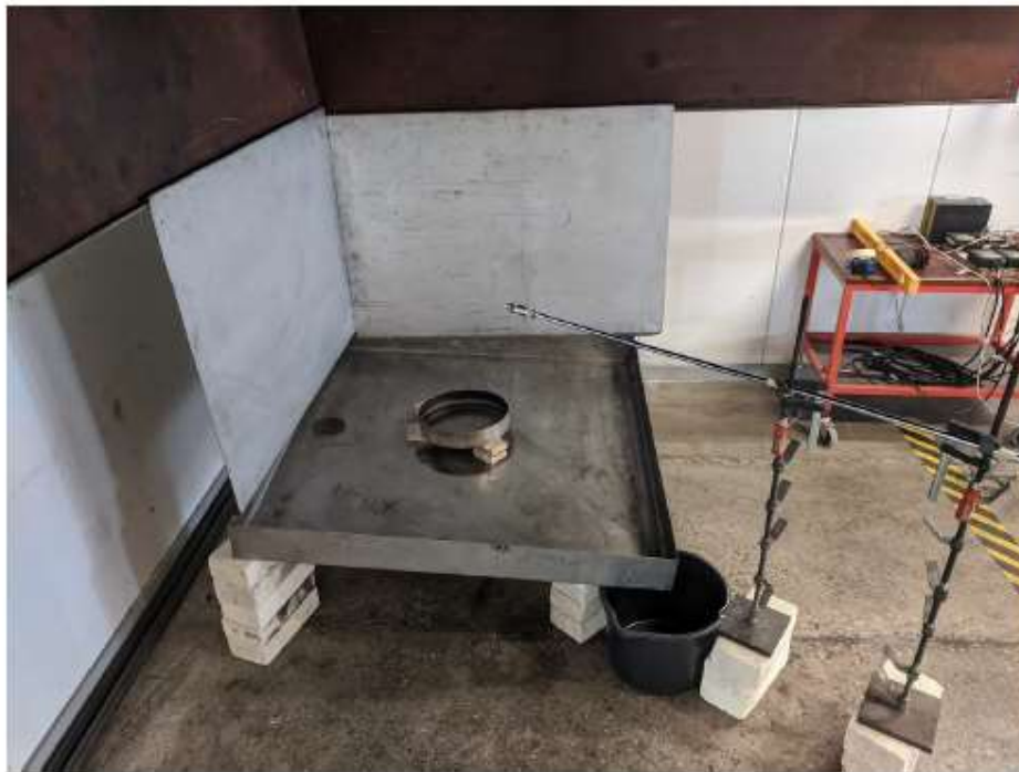
Figure 3. Experimental Apparatus – General Arrangement (Note: this image does not show the outer spill pan or the clamps used to secure the steel plates to the extraction hood)
