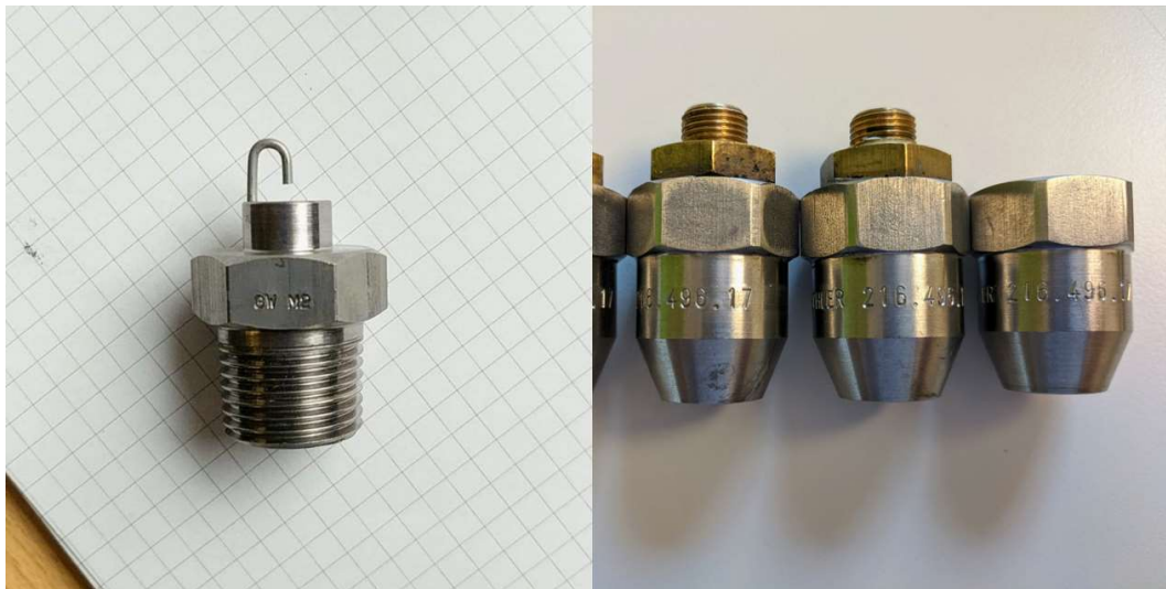
Figure 9 – Mist nozzles utilised GW Sprinkler AS, GW M2 (left) and Lechler Series 216.496 (right)
