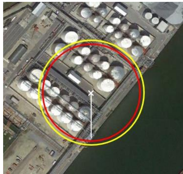
Figure 25. Case study explosion contours, rupture case
