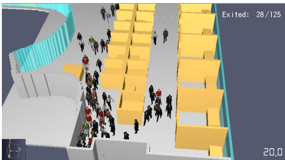
Fig. 15 Illustration of an evacuation simulation at 20s with Pathfinder
