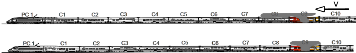
Figure 12 Fire on carriage 9; unidirectional ventilation (top), natural ventilation (bottom)
