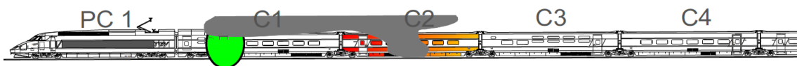
Figure 5 Fire on C2 affecting a cross passage in a controlled stop situation
