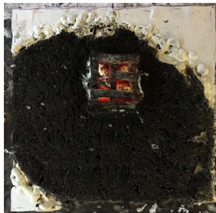
Figure 30 The fire spread in Test 15. The width was wide enough to support the fire spread until the end of the membrane length
