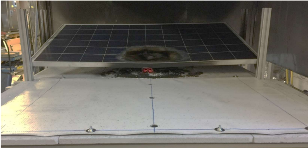
Figure 17 The fire spread in Test 23. The fire did not propagate outside the panel, while the membrane under the PV panel burned completely. The panel did not crack during the experiments; however, deformation of panels was observed during the tests
