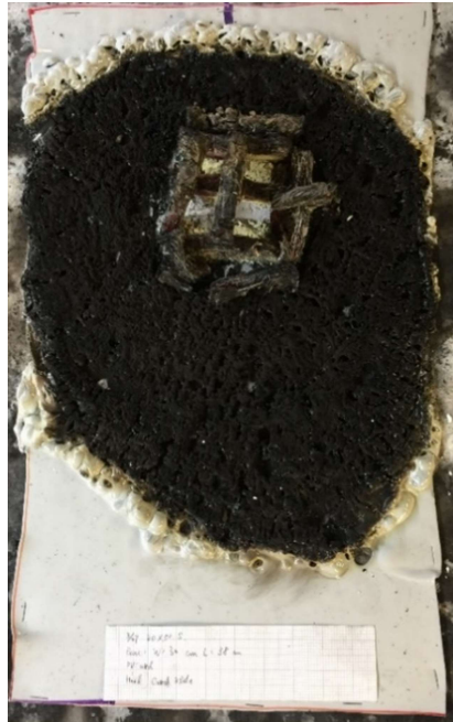
Figure 29 The fire spread in Test 14. The fire only spread 38.5 cm in all 50 cm length. It is assumed that the heat flux reduced when the fire spread to the end of membrane width, making the burning decreased in width at end side of fire spread. The spread of fire will be further discussed in Chapter 4
