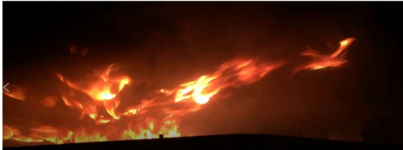
Figure 19 A picture of the fire burning on the backside of PV panels (Test 24). The flame propagated on the backside of the PV panel. The flame extended longer much than the membrane size, and the fire spread rapidly on the backside. The fire also burned more severely when new PV panels were used in the tests
