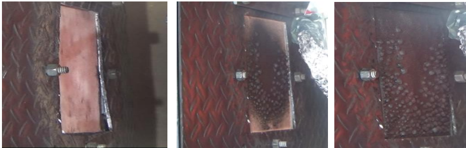
Figure 5. 5: Images of the intumescence process until total swelling activation of thin intumescent coating.
