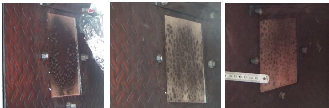
Figure 4. 1: Discrete swelling activation spots [HF_35_2] [7:30 minutes], [HF_25_1] [11 minutes] and [HF_16][21 minutes].
