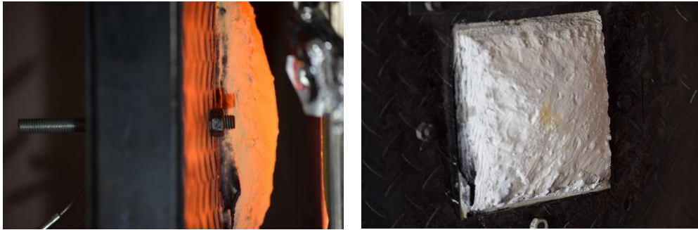
Figure 4. 20: Intumescent coating after stepwise heating increase.
