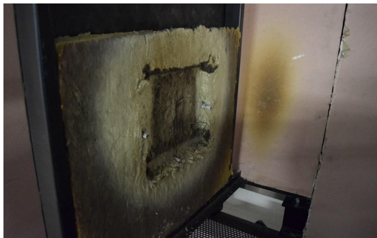
Figure 3. 13: Rockwool insulation filling the gap inside the sample holder.
