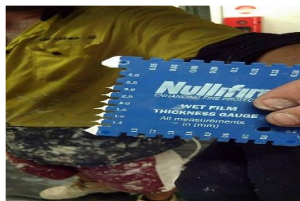
Figure 3. 4: Wet film thickness gauge comb.
