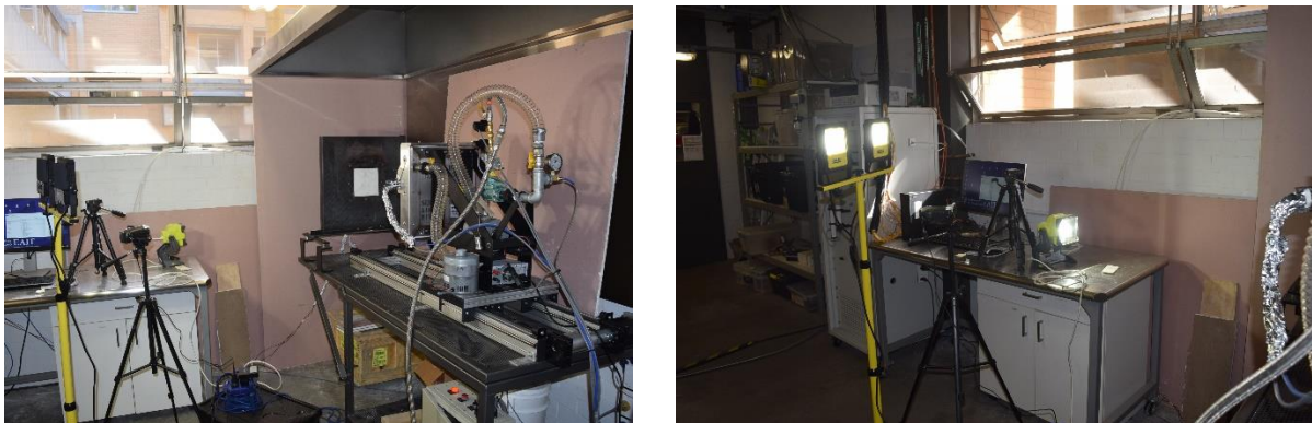
Figure 3. 15: Cameras and LED Lights used in the tests.
