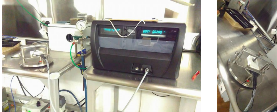
Figure 3. 7: Hot-disk instrument at the university of Queensland-Australia.
