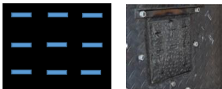
Figure 4. 17: Nine different measuring points throughout the coating.
