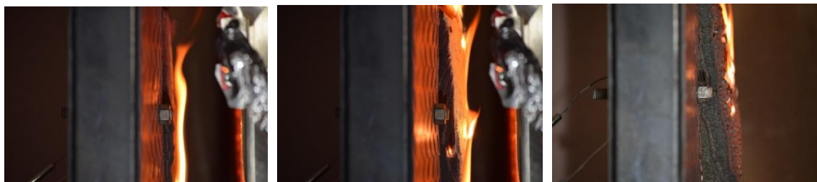
Figure 5. 9: Flame appearing over the surface of the coating from different tests.
