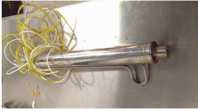
Figure 3. 10: Water Cooled Schmidt-Boelter.
