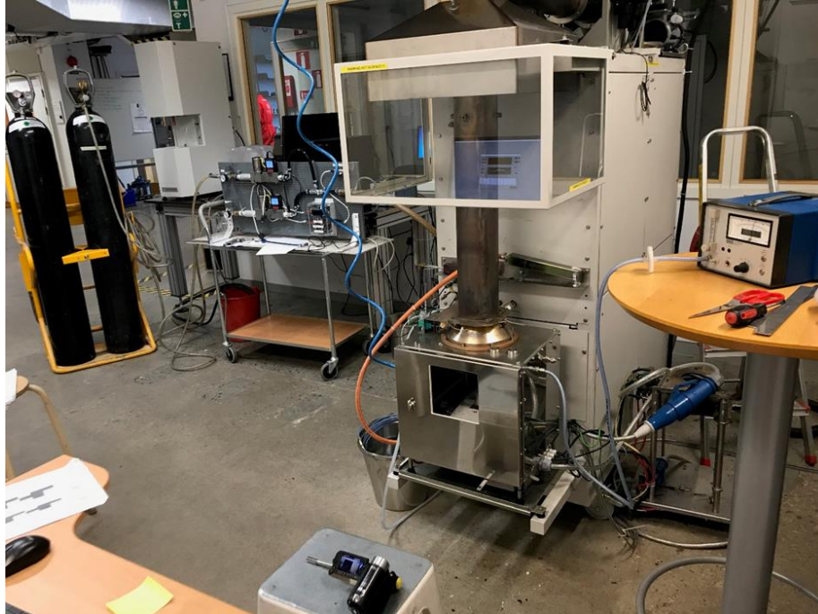
Figure 12 Entire CACC setup (N 2 cylinders and flow control on left of image and O 2 analyser on the right)
