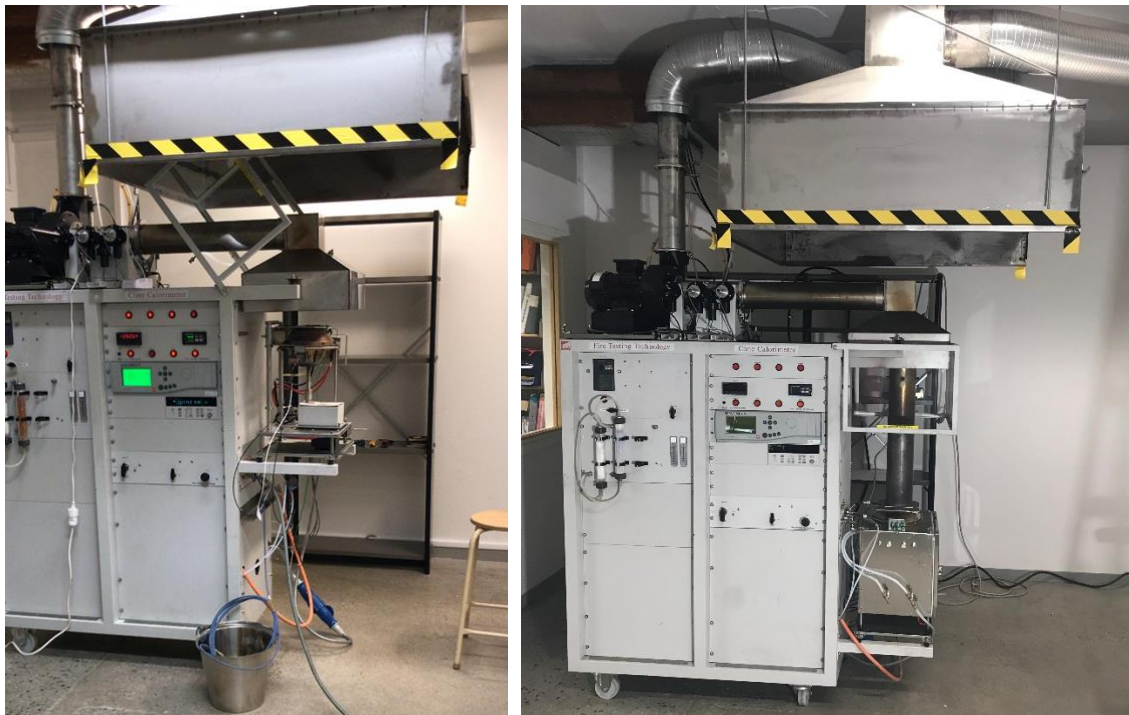
Figure 9 CC apparatus (left) and CACC installation (right) at Lund University
