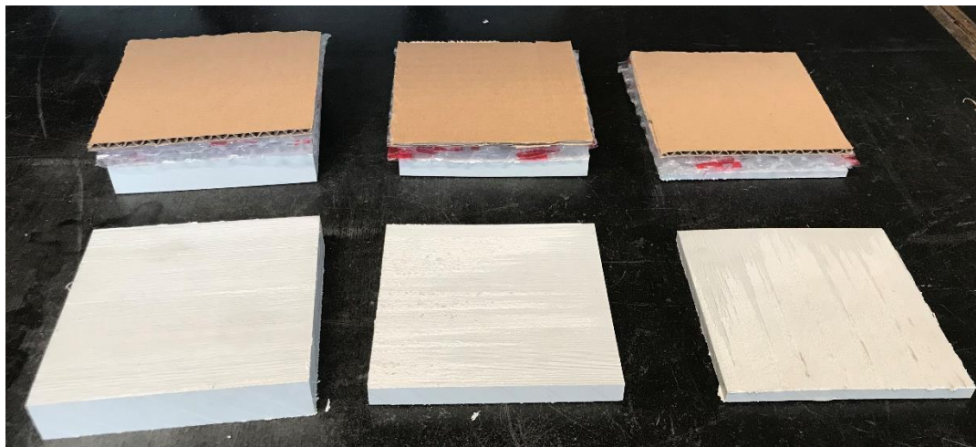
Figure 10 Thicknesses of pure ABS and composite samples
