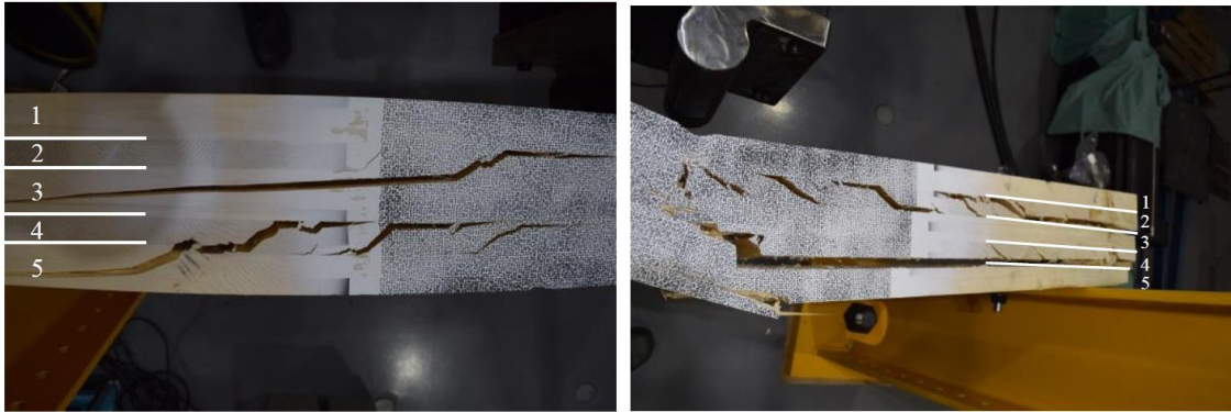
Figure 10. Failure mode change in the beam tested in three-point test. Timber failure at ambient temperatures (left) and bond line failure at elevated temperatures (65-80C, right) [26]
