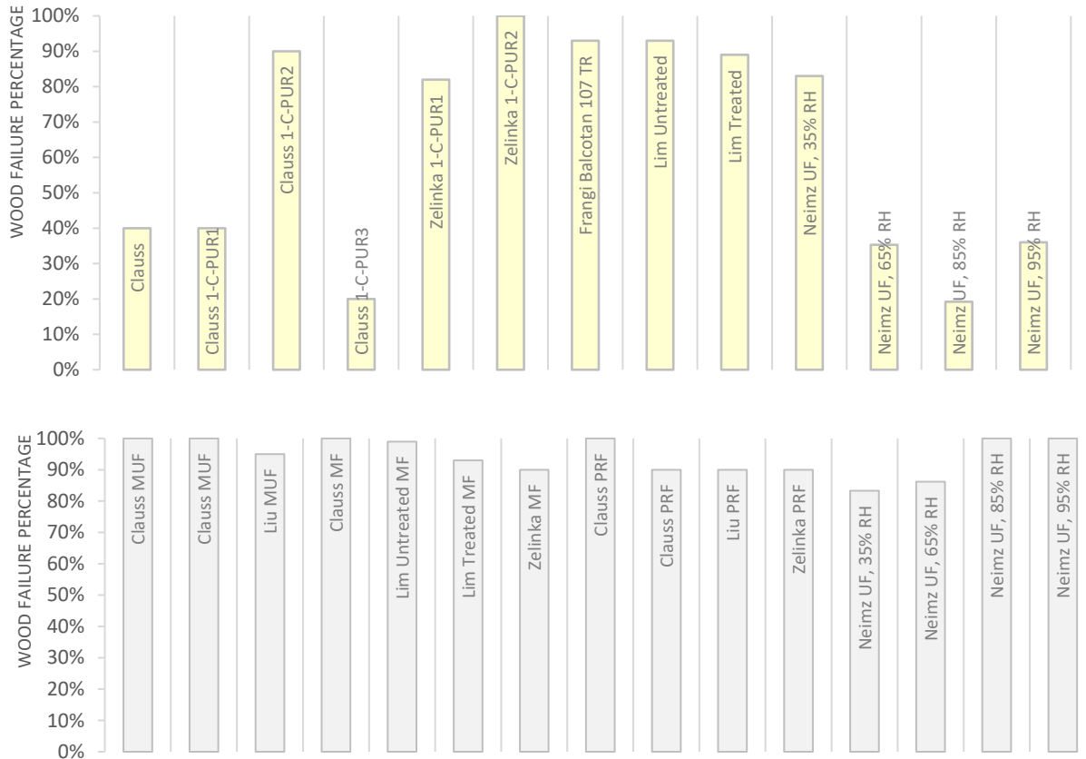
Figure 16. Wood failure percentage for different Polyurethanes (upper) and Formaldehydes (lower) at 20°C, adapted from Clauß et al [22], Niemz et al. [29], Frangi et al. [45], Clauß et al [51], Liu et al. [88], Zelinka et al. [127] and Lim et al. [141]
