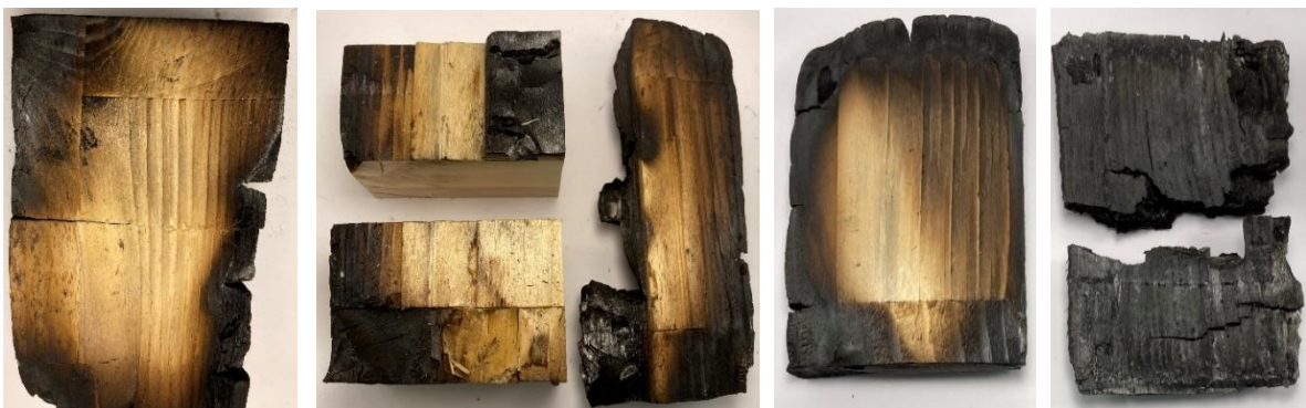
Figure 42. Delamination: Timber failure: sliding of fibres in the first lamella. From left to right: B9, B14, A14
