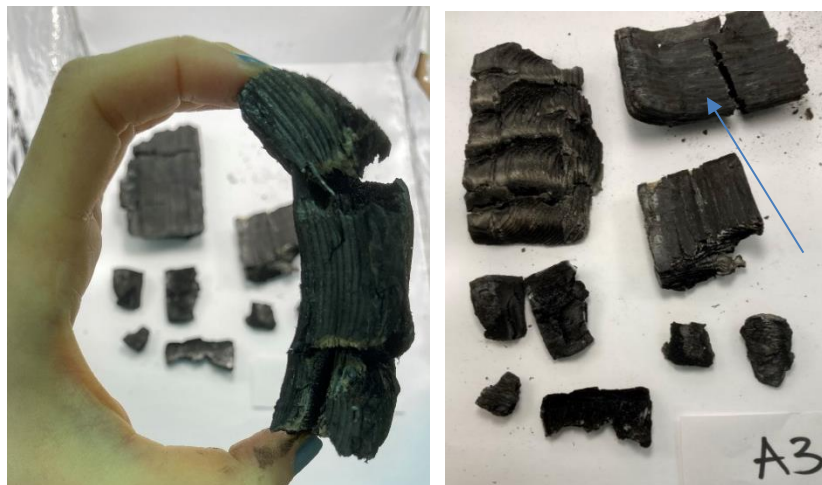
Figure 47. Buckled char fall-off residue
