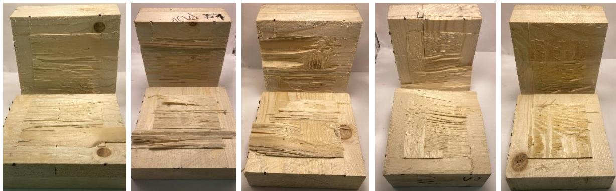
Figure 30. Failure modes for ambient tests. From left to right: High wood failure percentage A2, B1, B2, C1; Partial adhesive cohesion failure C2.
