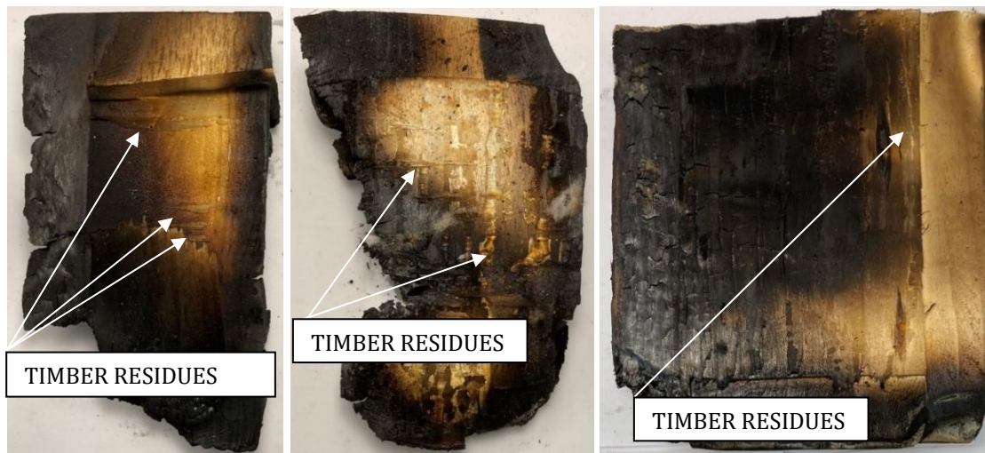
Figure 41. Delamination: Adhesive-timber failure: bond-line interface with timber residues from the second lamella. From left to right: PUR2 B12; MUF C7, C8.
