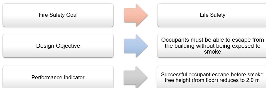
Figure 4.7: Fire safety goal, design objective and performance indicator for the office building case study
