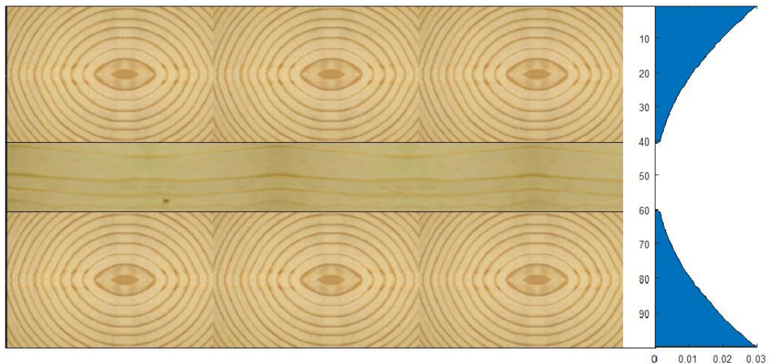
Figure 24 Influence of each layer to the total bending stiffness for the three- layer configuration
