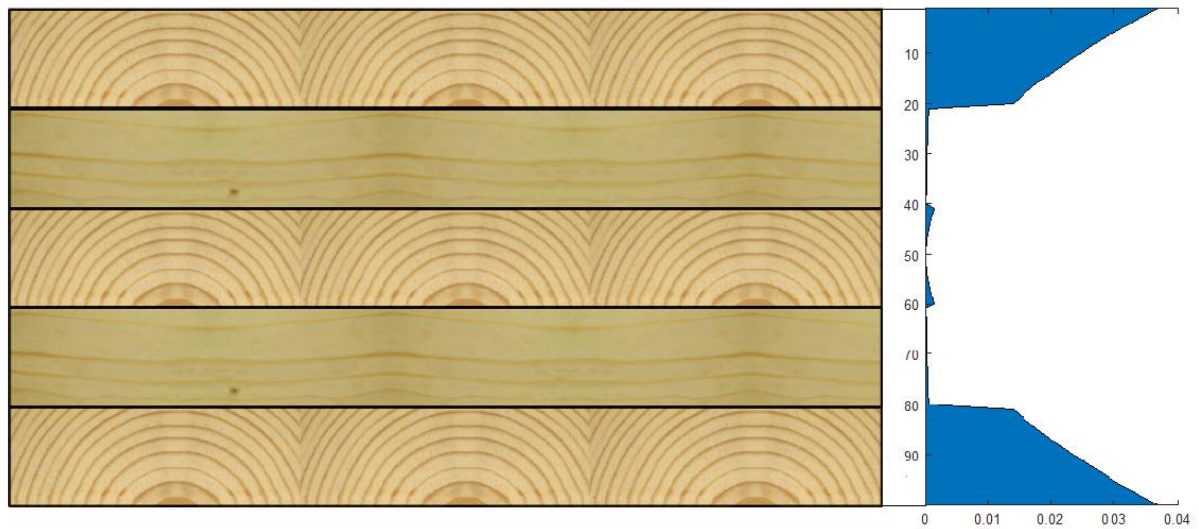
Figure 23 Influence of each layer to the total bending stiffness for the five layer configuration
