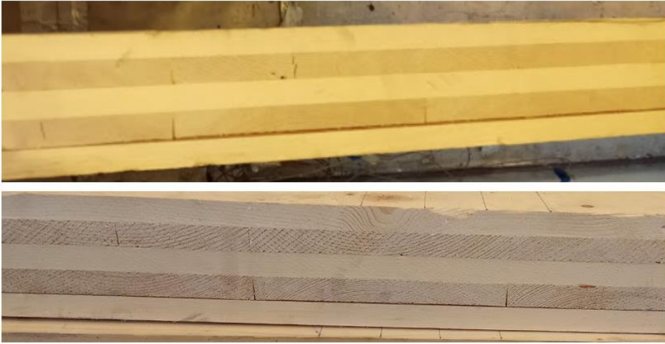
Figure 41 Delamination of layers observed on the bottom side of the beam used in Test 1 after cooling (both sides of the beam)
