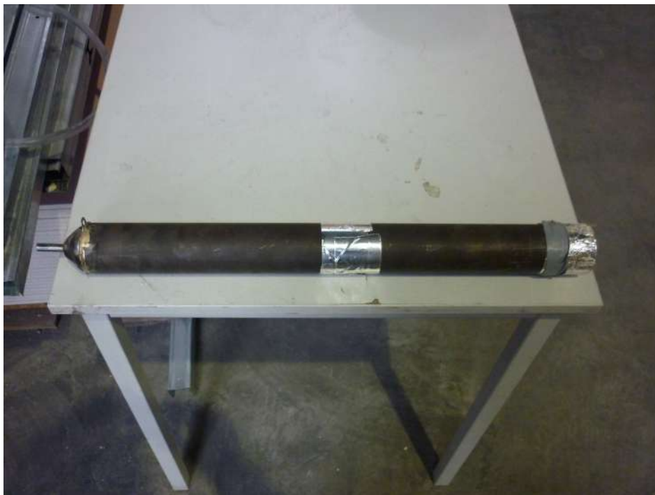
Figure 6.10: This is how the homemade divergent looks like, this will be attached on the model.
