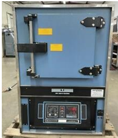
Figure 19: Furnace used to heat OSB3 samples
