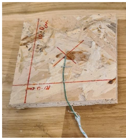
Figure 21: Attaching thermocouple to the center of OSB3 sample
