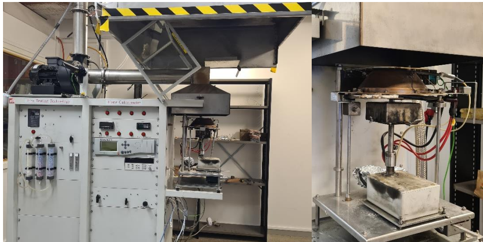
Figure 17: Set-up of the cone-calorimeter apparatus
