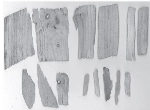
Figure 7: Strand types in OSB Reproduced from [20] with the permission from Elsevier
