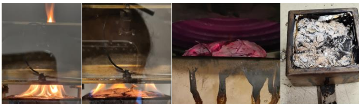
Figure 25: OSB3 sample during cone calorimeter test and afterwards
