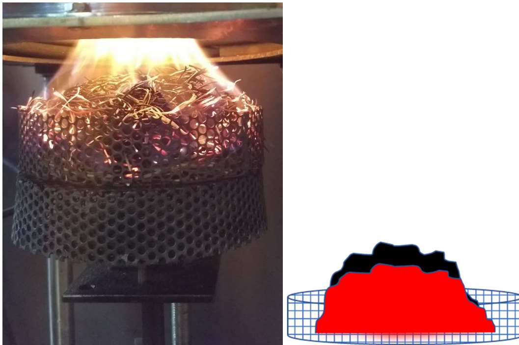
Figure 13: (Left) Test setup. (Right) Visualisation of samples lifting up while burning.
