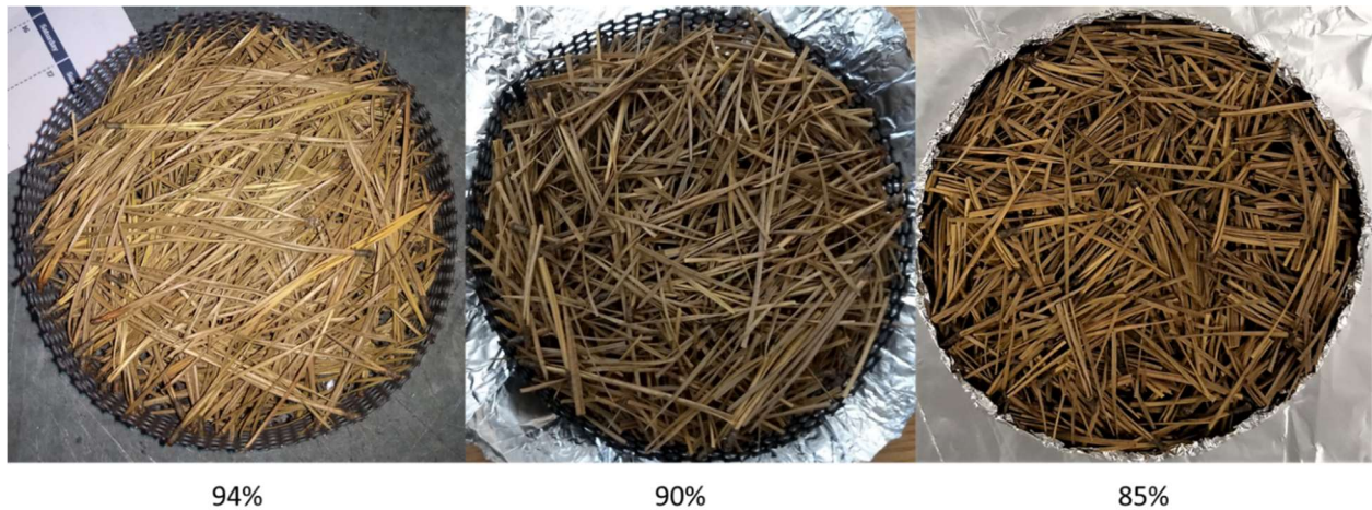
Figure 11: Samples of 94%, 90% and 85% porosities. First sample is ready for test. Second is while the aluminium foil is being removed and third is just when it was taken out of the oven.
