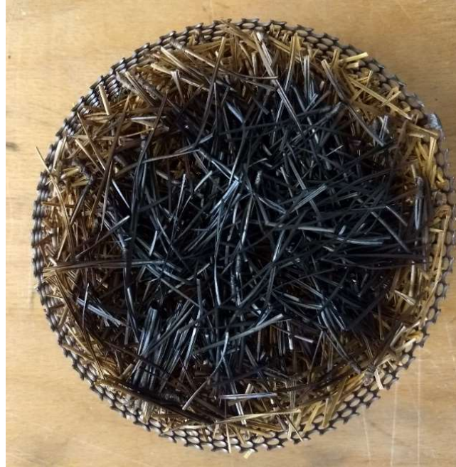
Figure 14: 85% porosity at 13.5 kW/m 2 (Area towards the edges are not charred)
