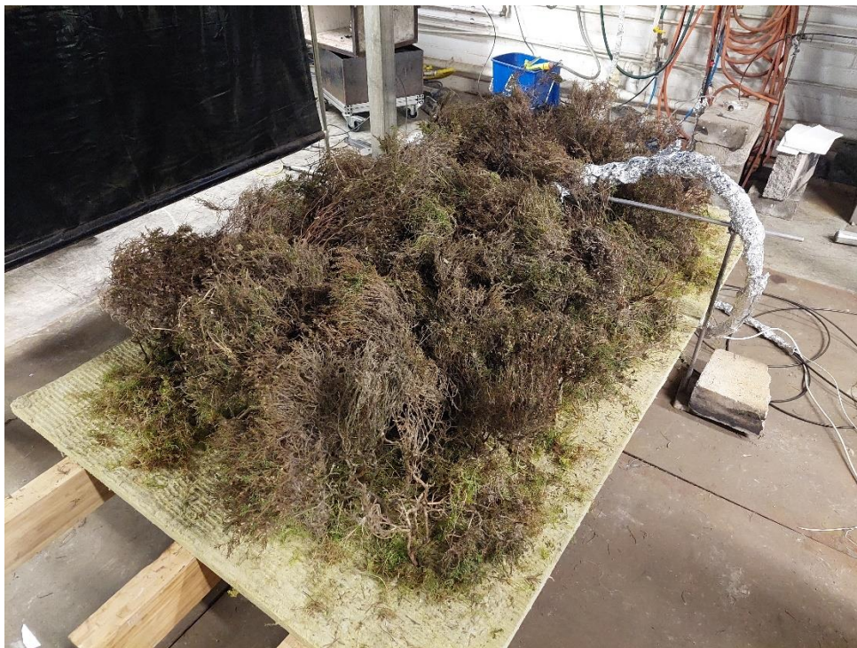
Figure 3. Example of an artificial fuel bed with moss layer.
