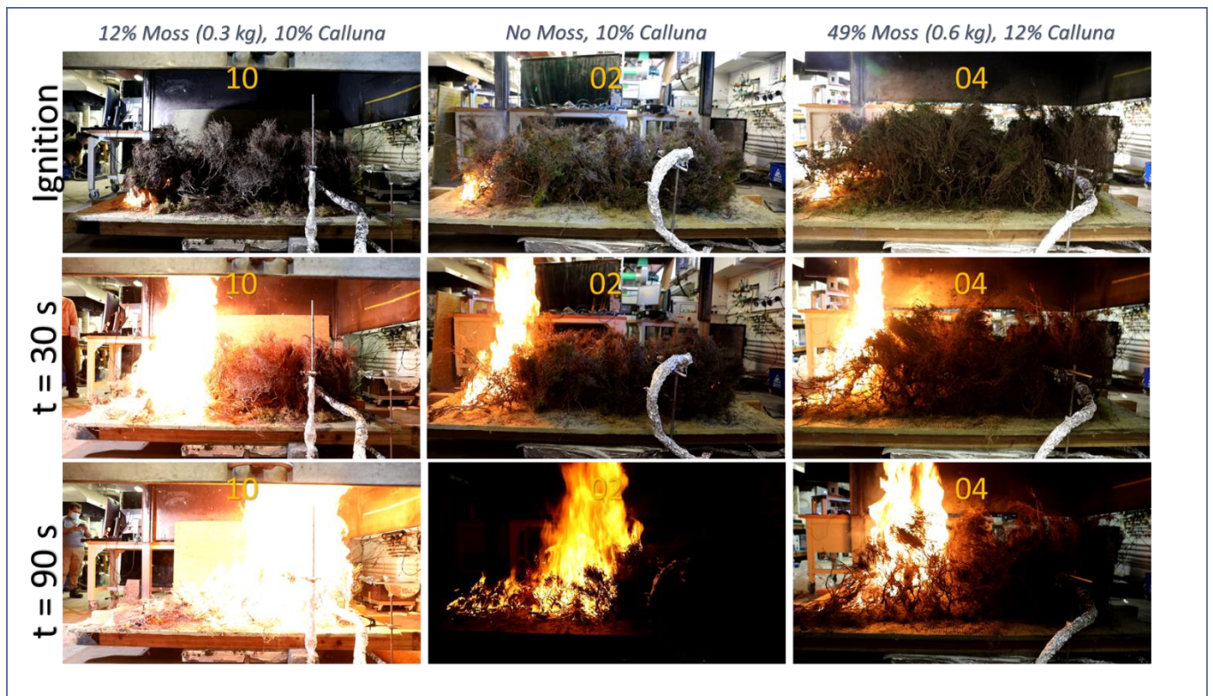
Figure 11. Experiments 10, 2 and 4; images taken right after the ignition, 30 seconds after the ignition and 90 seconds after the ignition. All the experiments had ~5 kg of Calluna fuel load.
