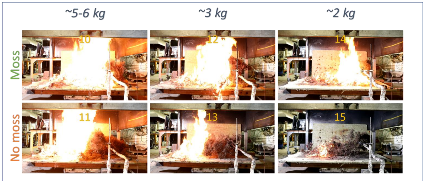
Figure 9. Experiments 10-15; images taken 75 seconds after the ignition.
