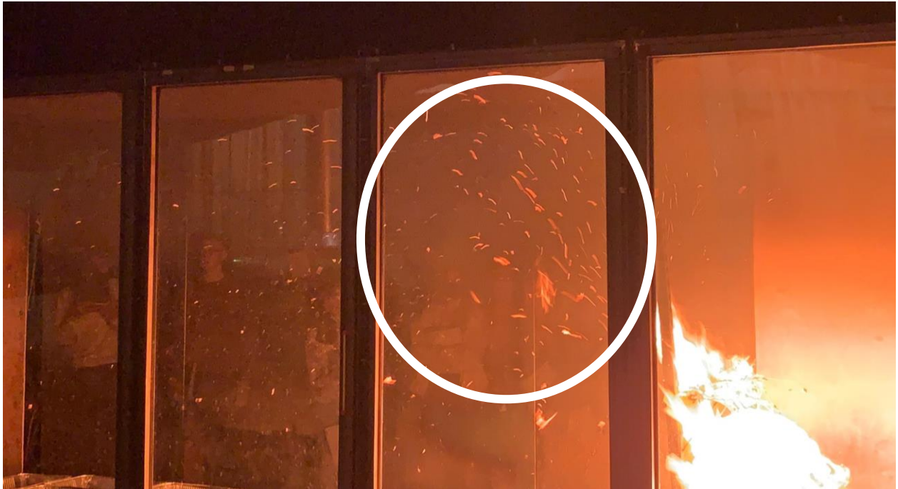
Fig. 22: Firebrands going up due to the fire-induced plume
