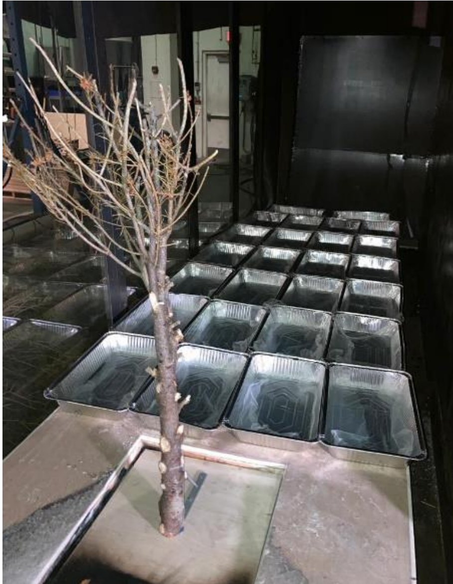
Fig. 9: Interior of the test section with the trunk setup and the pans layout
