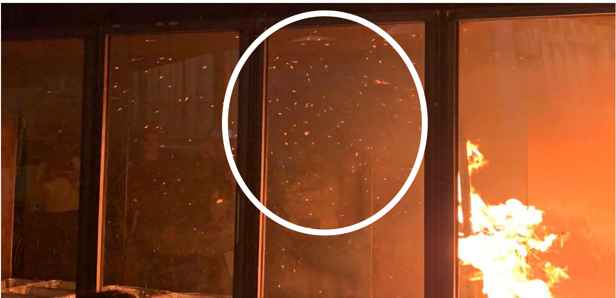
Fig. 23: Firebrands travelling inside the test section
