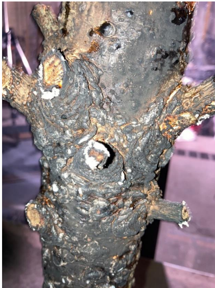
Fig. 21: Smouldering on the bark of Douglas Fir trunk
