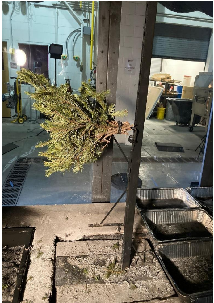
Fig. 6: Holder setup for experiments using branches
