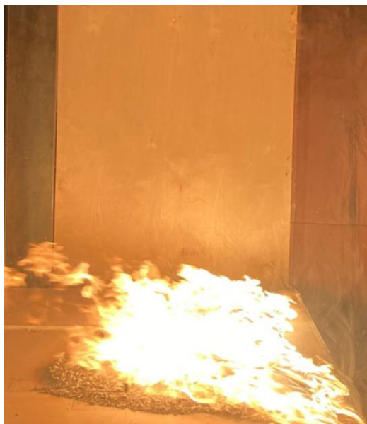
Fig. 13: Flame shape under 1 m/s wind velocity
