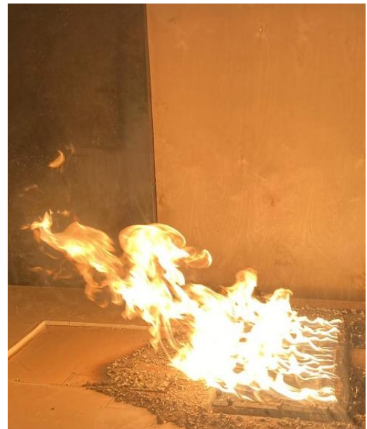
Fig. 14: Flame shape under 0.4 m/s wind velocity
