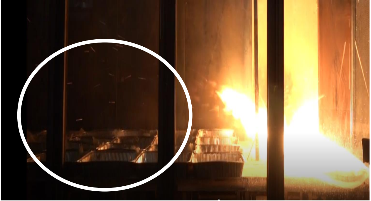
Fig. 37: Firebrand shower phenomenon from a 2 m/s branches test
