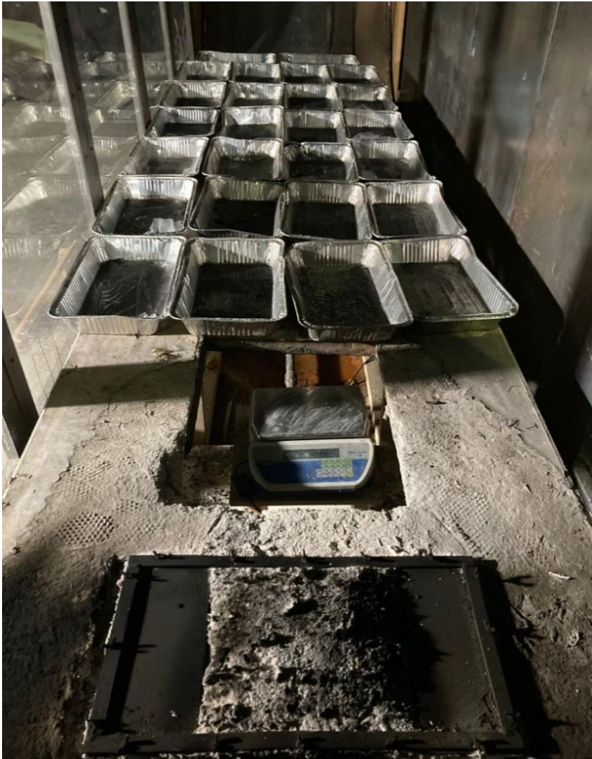
Fig. 8: Interior of the test section with the burner, the scale and the pans layout
