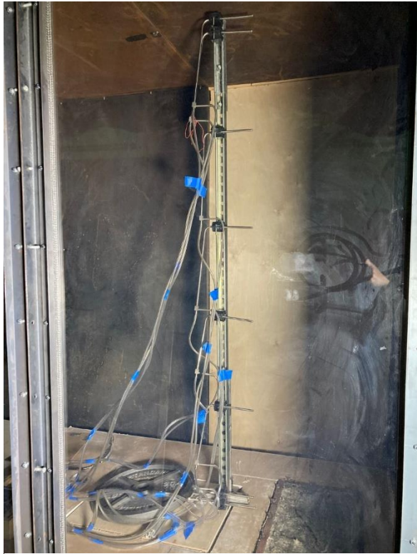
Fig. 12: Steel tree with Pitot tubes used for the characterization of the air flow
