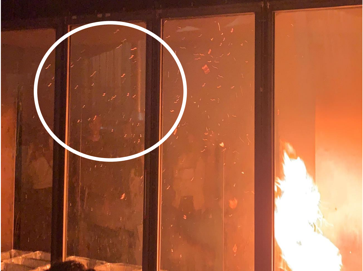
Fig. 24: Firebrands falling in the test section
