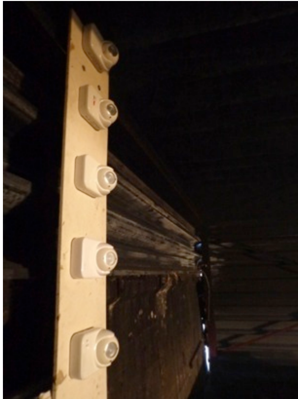
Figure 32: Smoke layer depth measurement experiments – OSID Array
