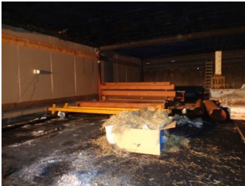
Figure 31: Smoke layer depth measurement experiments – Straw
