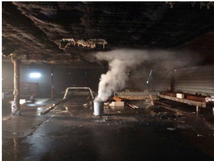
Figure 34: Smoke detection and localization experiments – Paper in metallic bin
