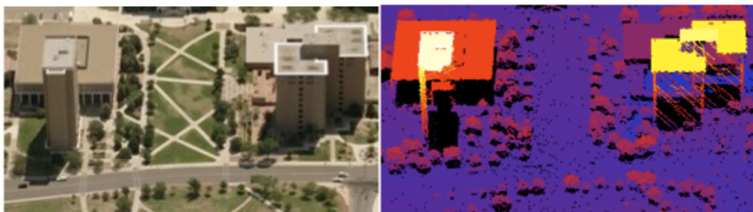
Figure 5: Height-encoded LIDAR image of an urban scene (Taken from [20])
