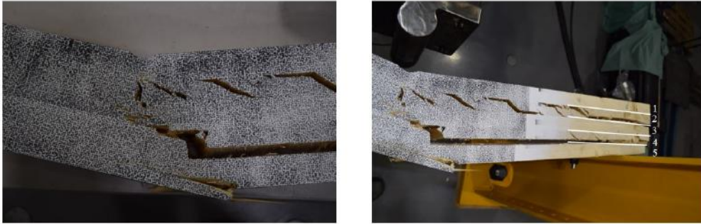
Figure 1.19: CLT beam after elevated temperature test: Beam centre with failure initiation location (left) Beam after failure (right) [17]
