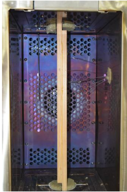
Figure 2.10: Sample with thermocouples placed for thermal penetration test
