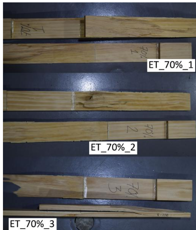
Figure 3.10: Delamination of samples at 70% loading
