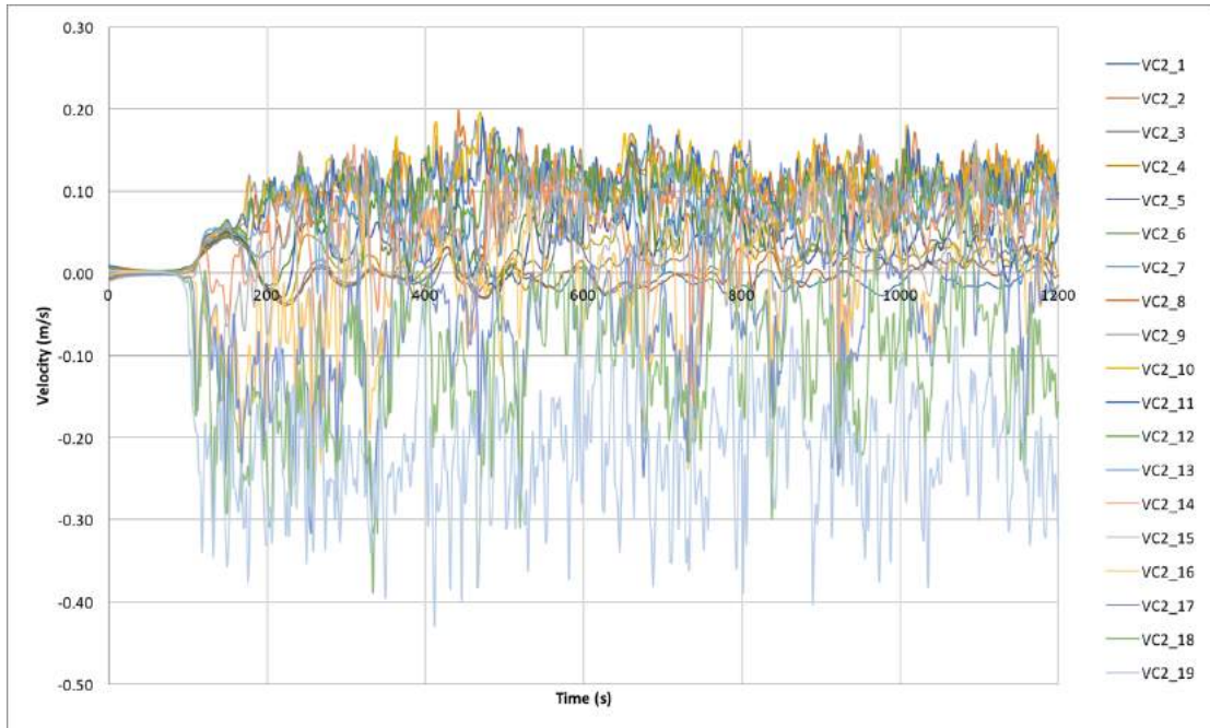
Figure C.3 Velocities along the Center Line of the Second Floor Compartment in M2
