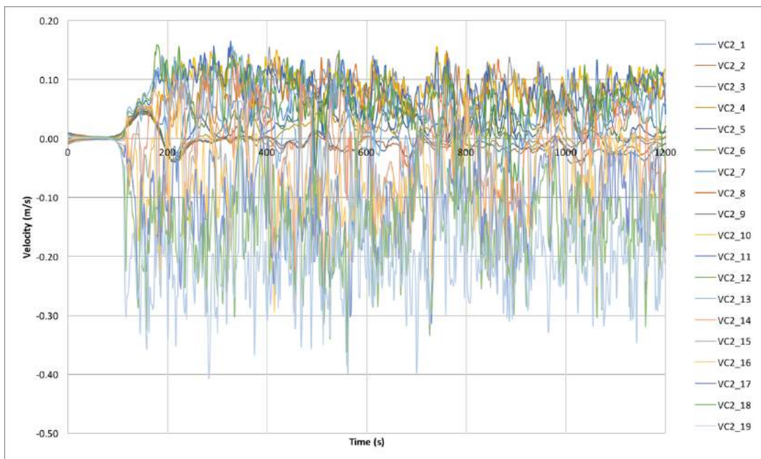
Figure C.12 Velocities along the Center Line of the Second Floor Compartment in M5
