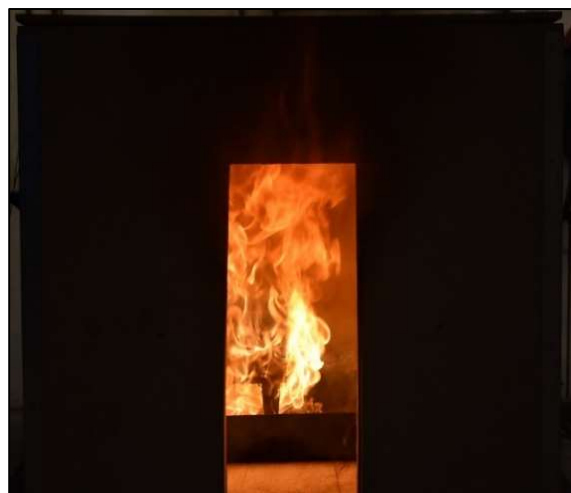
Figure 25. Case 2 with the Phenolic insulation showing a visual indication of a ventilation-controlled fire as flames shoot out of the compartment and thick black smoke is also observed.
