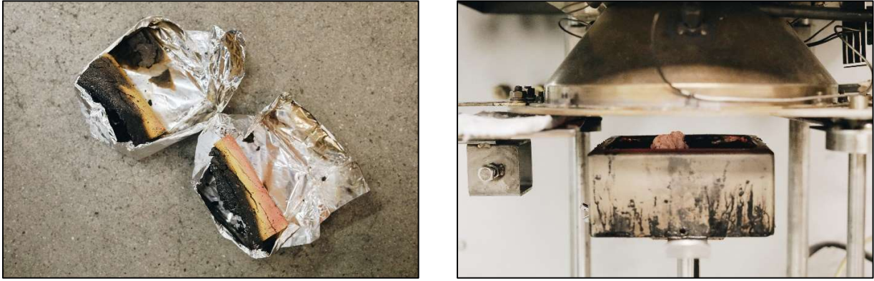
Figure 20. L: PIR and Phenolic insulation samples after burning. R: Remaining composite material after the cone test.
