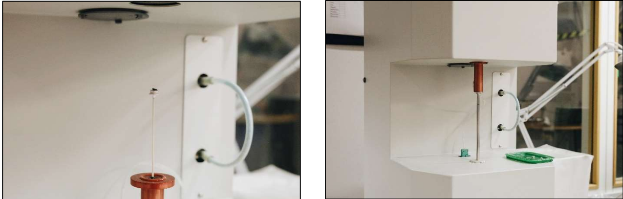
Figure 10. A sample of fabric is loaded into the ceramic crucible and tested in both Method A and B.
