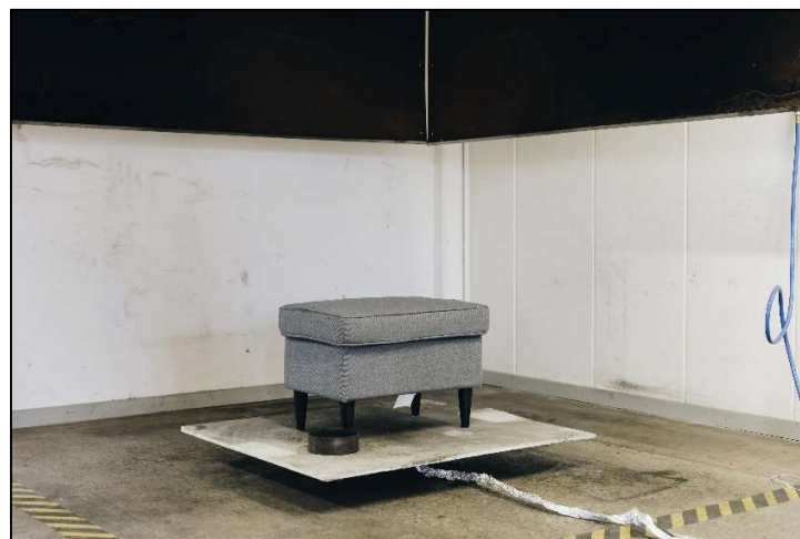
Figure 16. Experimental set-up of the open calorimeter test conducted in the LTH Fire Laboratory.
