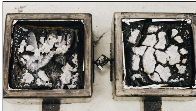
Figure 22. Phenolic insulation after the tests showing cracks.
