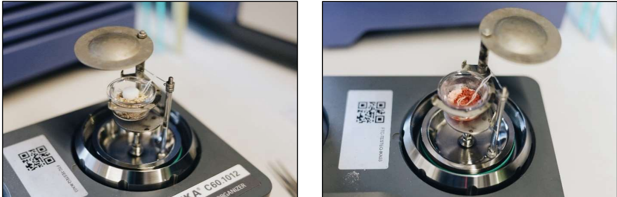
Figure 11. Bomb calorimeter set-up of chipboard shavings plus benzoic acid tablet (L) and phenolic insulation powder with paraffin oil (R), and cotton thread.
