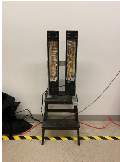
Figure 9 - The thermal radiation device
