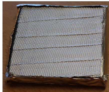
Figure 38: Sample B-C-1 of epoxy composite Figure 39: Sample B-C-1 of epoxy composite type 2 after test in cone calorimeter
