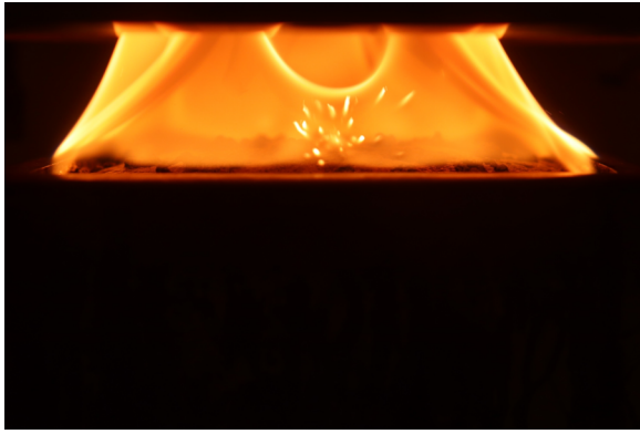
Figure 40: Sample C-C-1 of fresh epoxy resin during the test in the cone calorimeter
