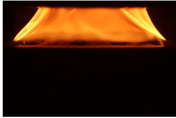
Figure 41: Sample C-C-1 of epoxy composite type 2 during the test in the cone calorimeter
