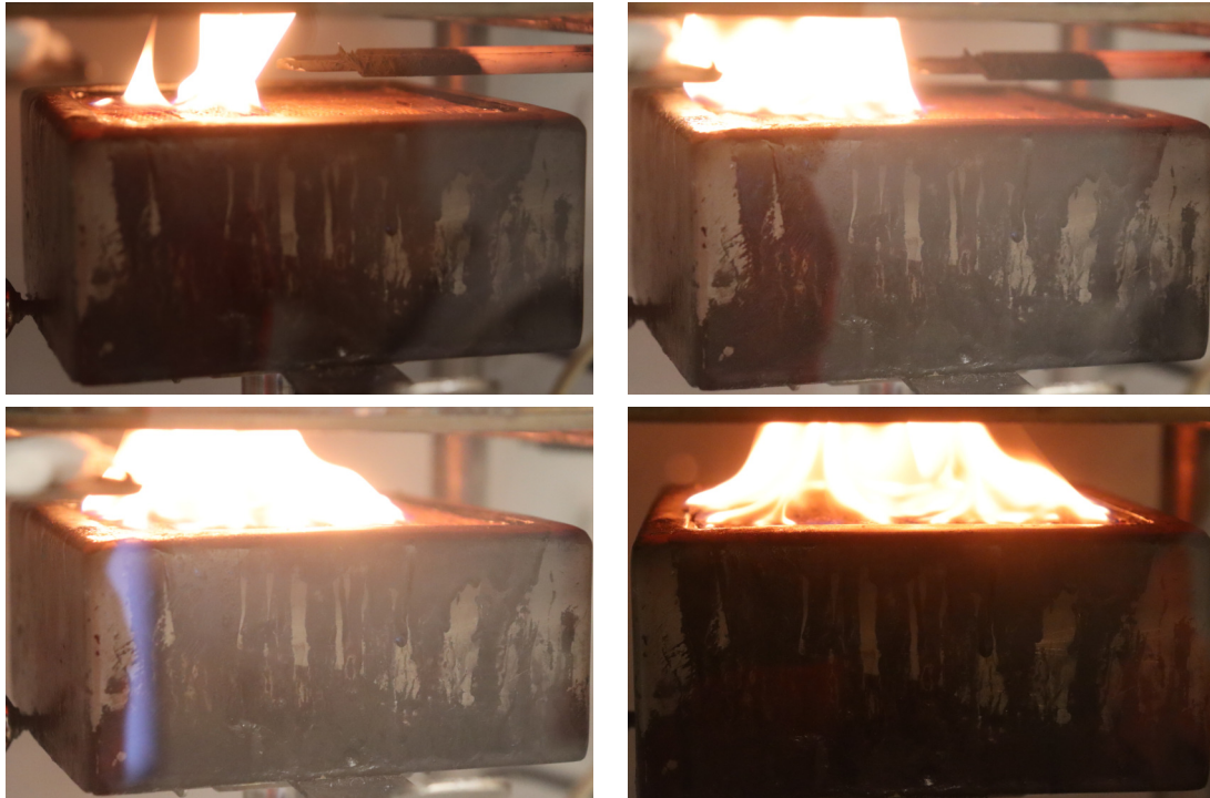
Figure 37: Sample B-C-1 during test in cone calorimeter
