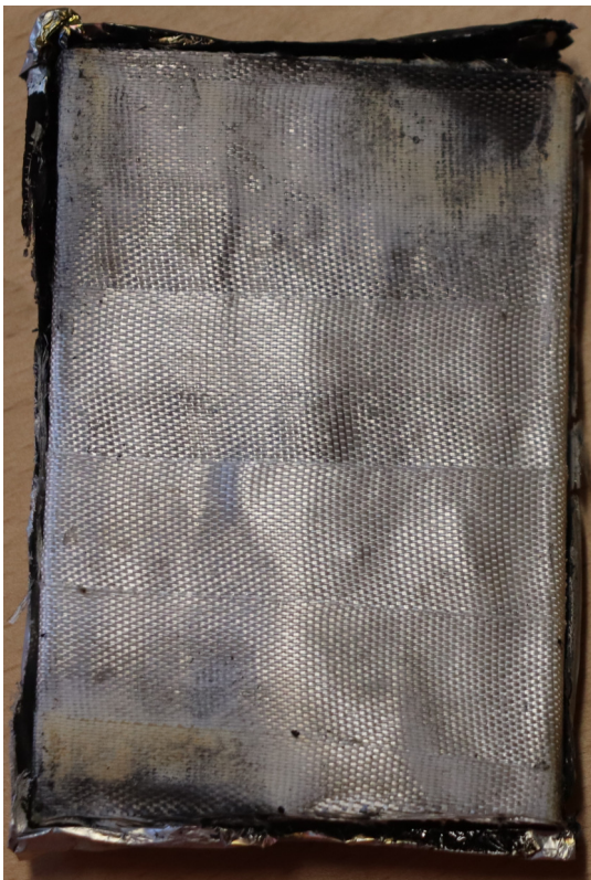
Figure 33: Sample A-C-1 of epoxy composite type 1 after test in cone calorimeter. Upper face Figure 34: Sample A-C-1 of epoxy composite type 1 after test in cone calorimeter. Bottom face
