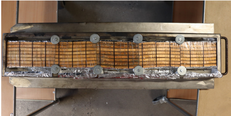
Figure 64: Sample B-L-1 for test 2 of epoxy composite type 2 in the sample holder for the LIFT. The sample consists of five segments with gaps between them.
