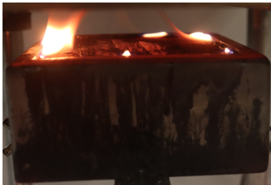
Figure 38: Sample B-C-1 of epoxy composite Figure 39: Sample B-C-1 of epoxy composite type 2 after test in cone calorimeter
