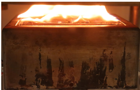
Figure 35: Sample A-C-1 of epoxy composite type 1 during test in the cone calorimeter
