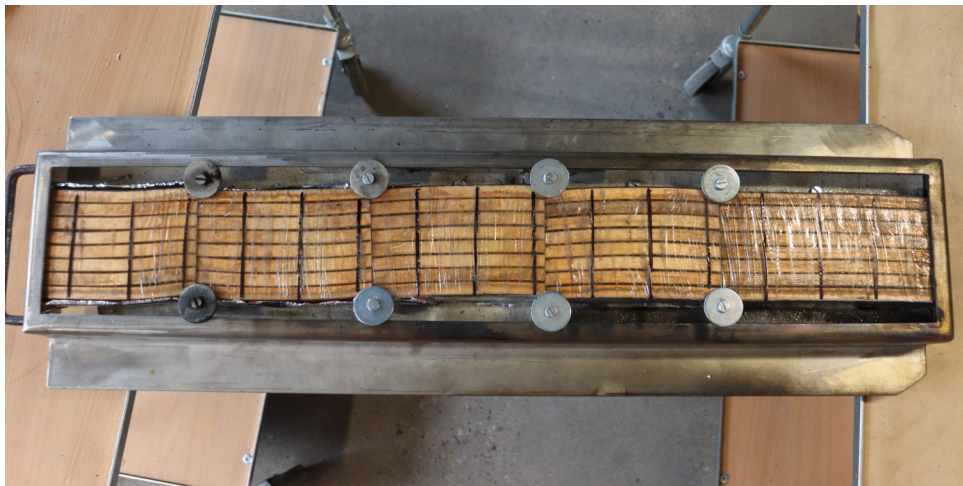
Figure 65: Sample B-L-2 for test 4 of epoxy composite type 2 in the sample holder for the LIFT. The sample consists of five segments with gaps between them.
