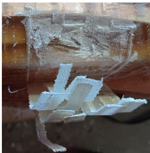
Figure 15: Appearance of epoxy resin type 2 from Magnetic coil type 2, after removing the fiber glass tape
