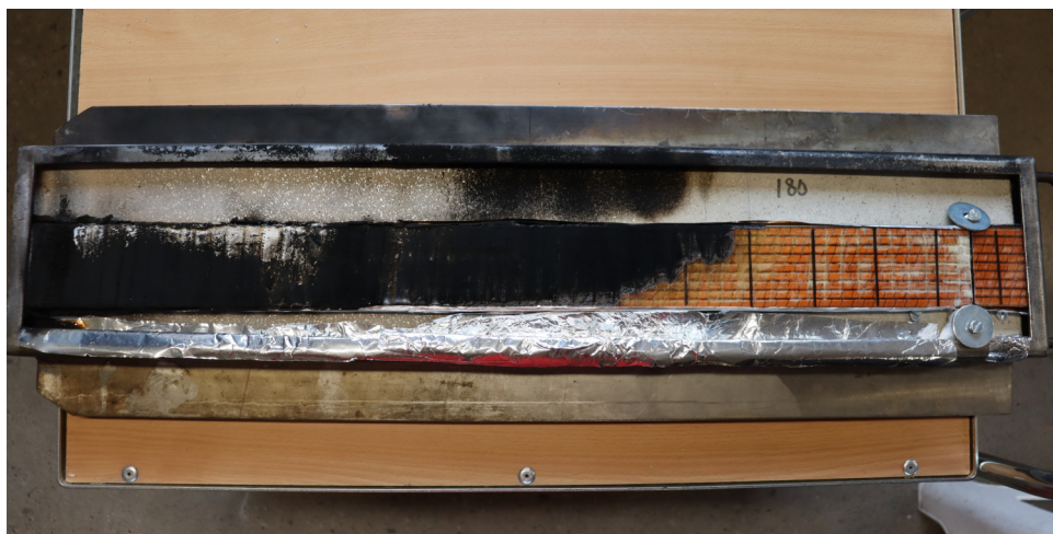
Figure 70: Sample A-L-1 after test 1 of epoxy composite type 1 in the LIFT
