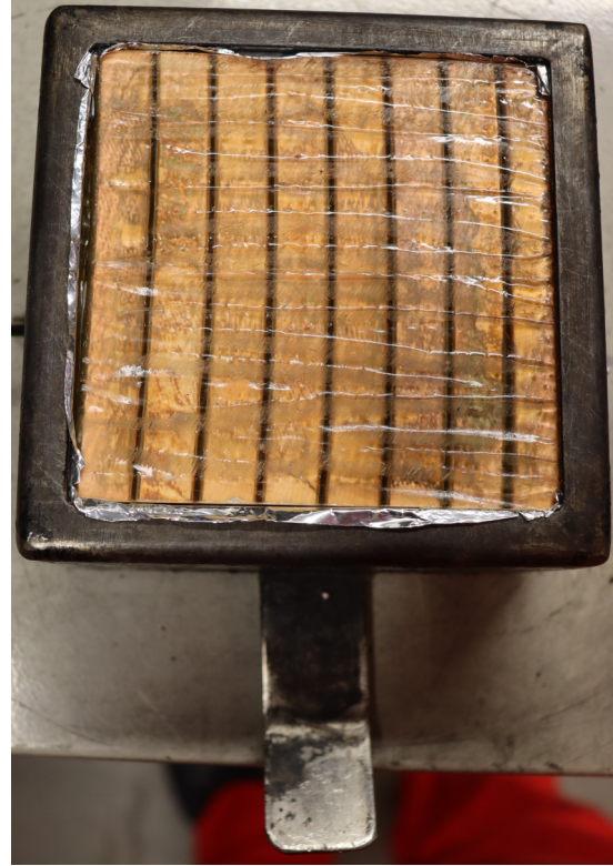
Figure 29: Sample A-C-1 of epoxy composite type 1 in sample holder for the test in the cone calorimeter
