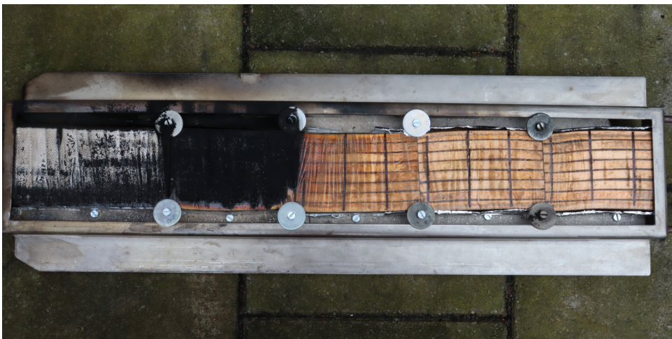
Figure 73: Sample B-L-2 after test 4 of epoxy composite type 2 in the LIFT
