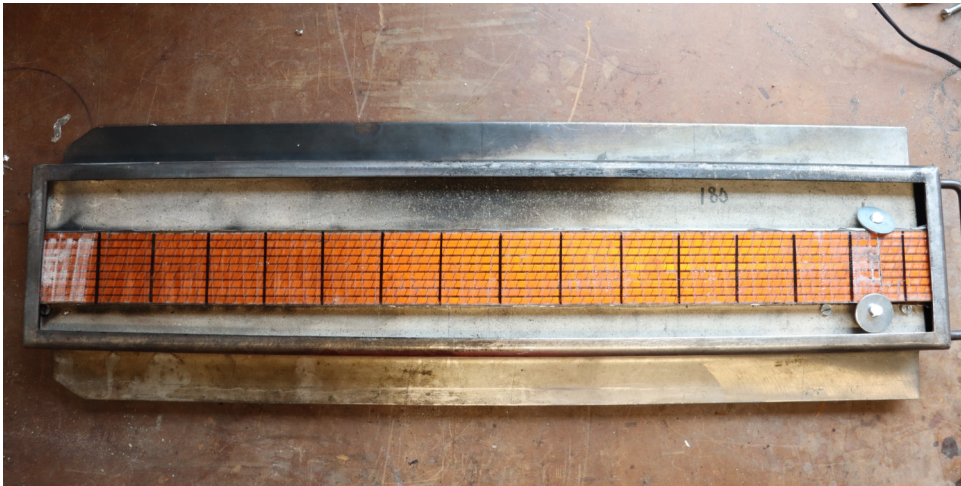
Figure 63: Sample A-L-2 for test 3 of epoxy composite type 1 in the sample holder for the LIFT. The gap between the two segments was located at the farthest end of the sample holder from the radiant panel and the external flame source
