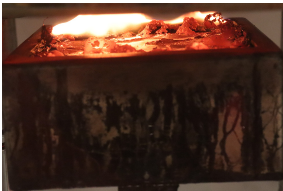
Figure 42: Sample C-C-1 of fresh epoxy resin during the test in the cone calorimeter
