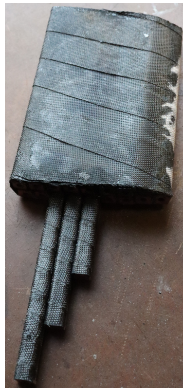
Figure 33: Sample A-C-1 of epoxy composite type 1 after test in cone calorimeter. Upper face Figure 34: Sample A-C-1 of epoxy composite type 1 after test in cone calorimeter. Bottom face
