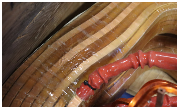
Figure 6: Magnetic coil type 2. Zoom in of accumulation of epoxy resin
