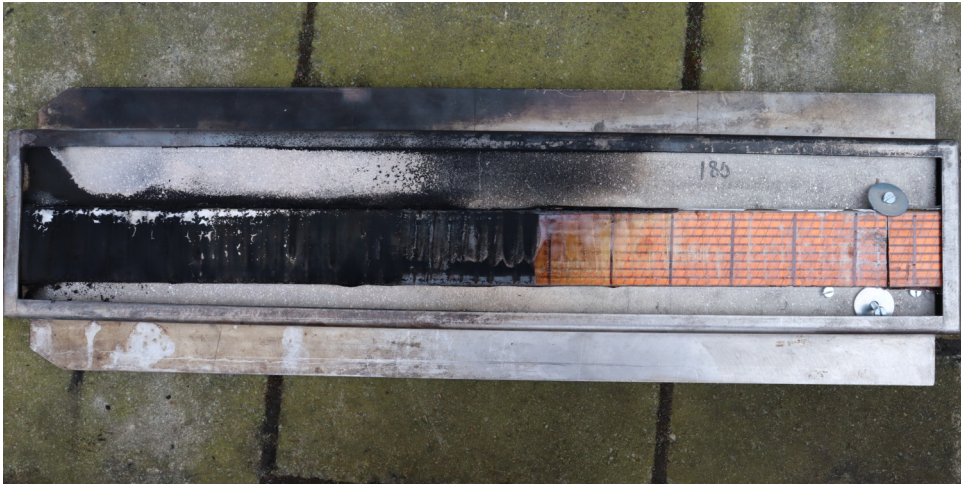
Figure 71: Sample A-L-2 after test 3 of epoxy composite type 1 in the LIFT
