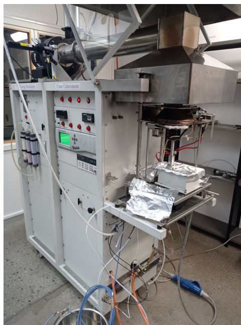
Figure 11: Illustration of cone calorimeter at Lund University
