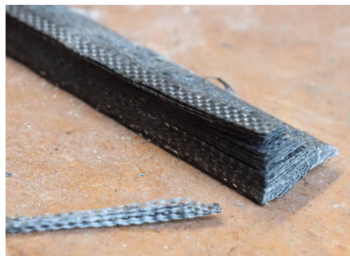
Figure 36: Sample A-C-1 of epoxy composite type 1 after test in cone calorimeter. Non-combustible filler material of magnetic coil type 1
