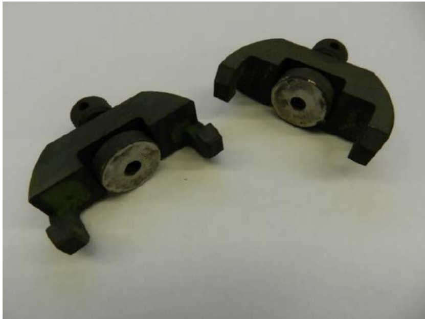
Figure 7: Fixers of the tensile machine.
