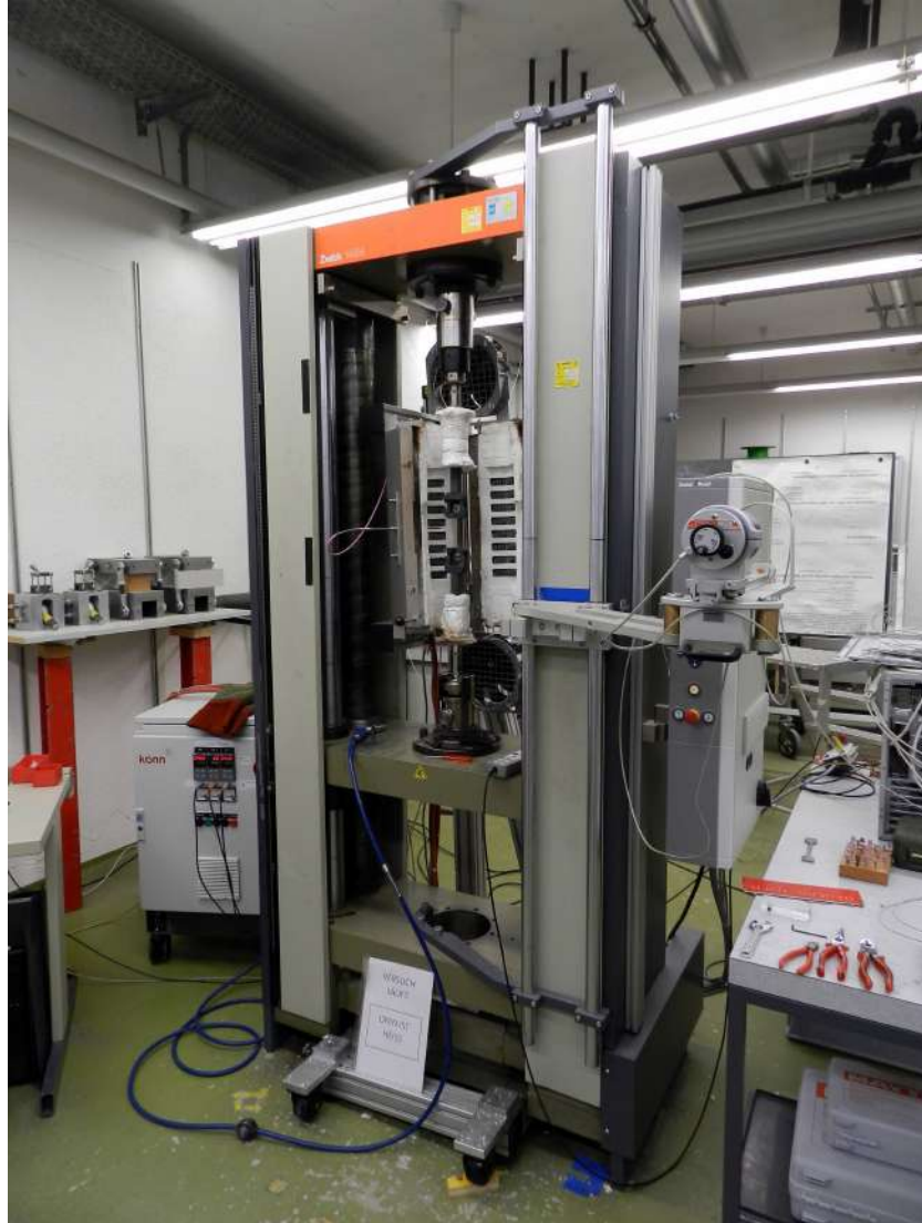
Figure 1: Tensile machine used to execute experiments.
