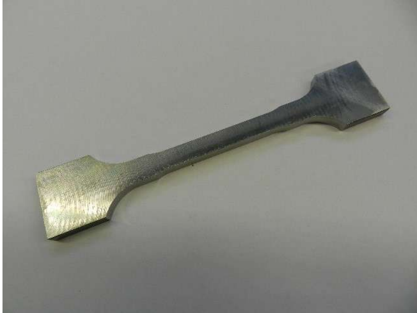
Figure 4: Test specimen made out of S960 high strength steel.
