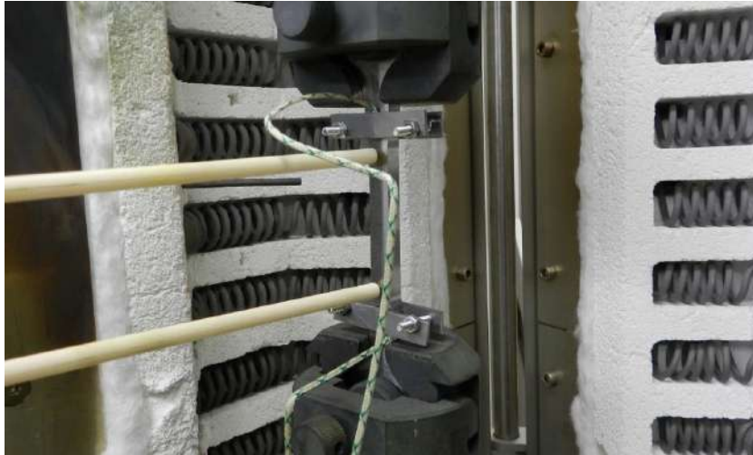
Figure 11: Sticks of the extensometer on the specimen.
